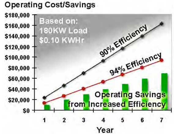
Figure 4. Operating efficiency in centralized vs. distributed systems results in considerable cumulative savings over the life of the UPS
